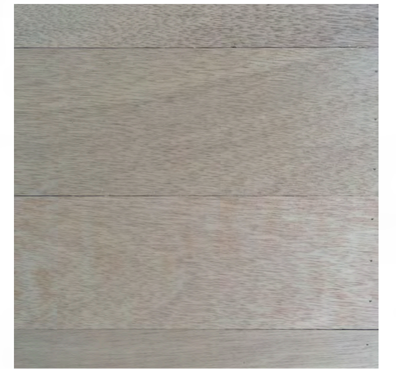
Plywood Boards Plywood is renewable and offered a breathable finish free of volatile organic compounds
