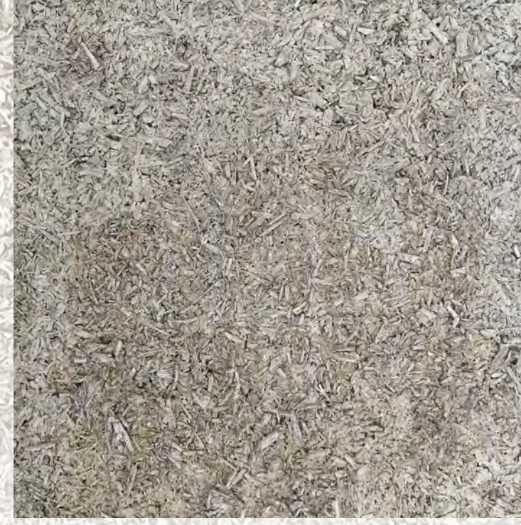
Hemp Insulation - Midwest Hemp Hemp Insulation - Midwest Hemp The use of Hemp Insulation was the main focus of the project. By mixing hurd, water, and lime to create this mixture.
