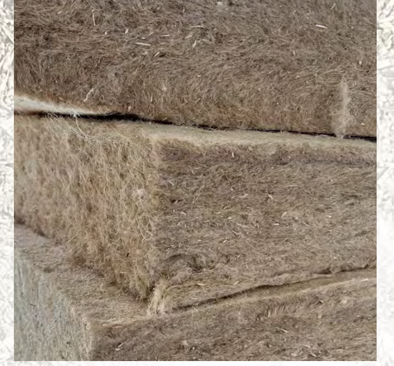
Hemp Wool - Hempitecture Hemp wool insulation was purchased to be installed in the floor and ceiling framing panels. This material is made from the fiber within the Hemp plant.
